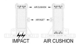
Impacting units provide the most force, but also produce higher noise levels. Air Cushioned (nonimpacting) models feature lower noise levels, but produce less force. When replacing an Impacting unit with an Air Cushioned, it may be necessary to use a larger model, or additional vibrators to achieve proper material flow.
