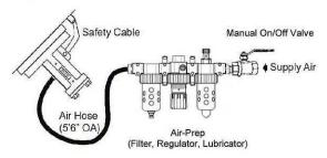
Single-unit manual installation for bins and hoppers is shown here for reference purposes.
